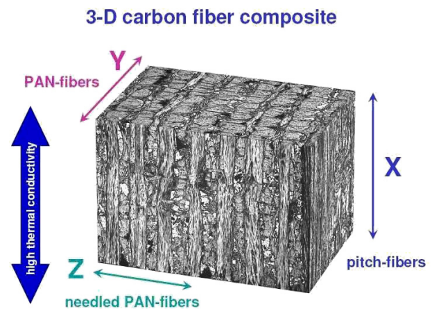
Figure 2. Fibre orientation in CFC-NB31 (courtesy of Dr Linke, Research Centre Juelich, IEF2).
